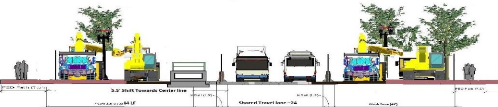
Cross-Section B - Looking East At Outbound Boarding Island Construction
