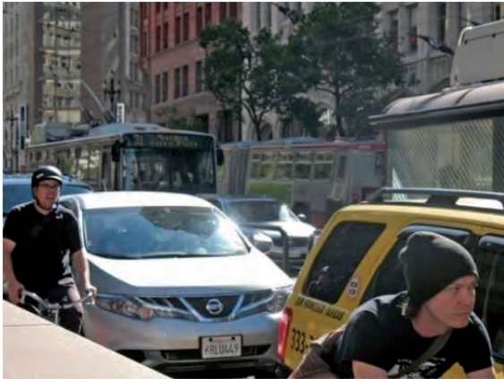
Figure 2.4.13: Bus Unable to Access Island Stop Because of Queue
