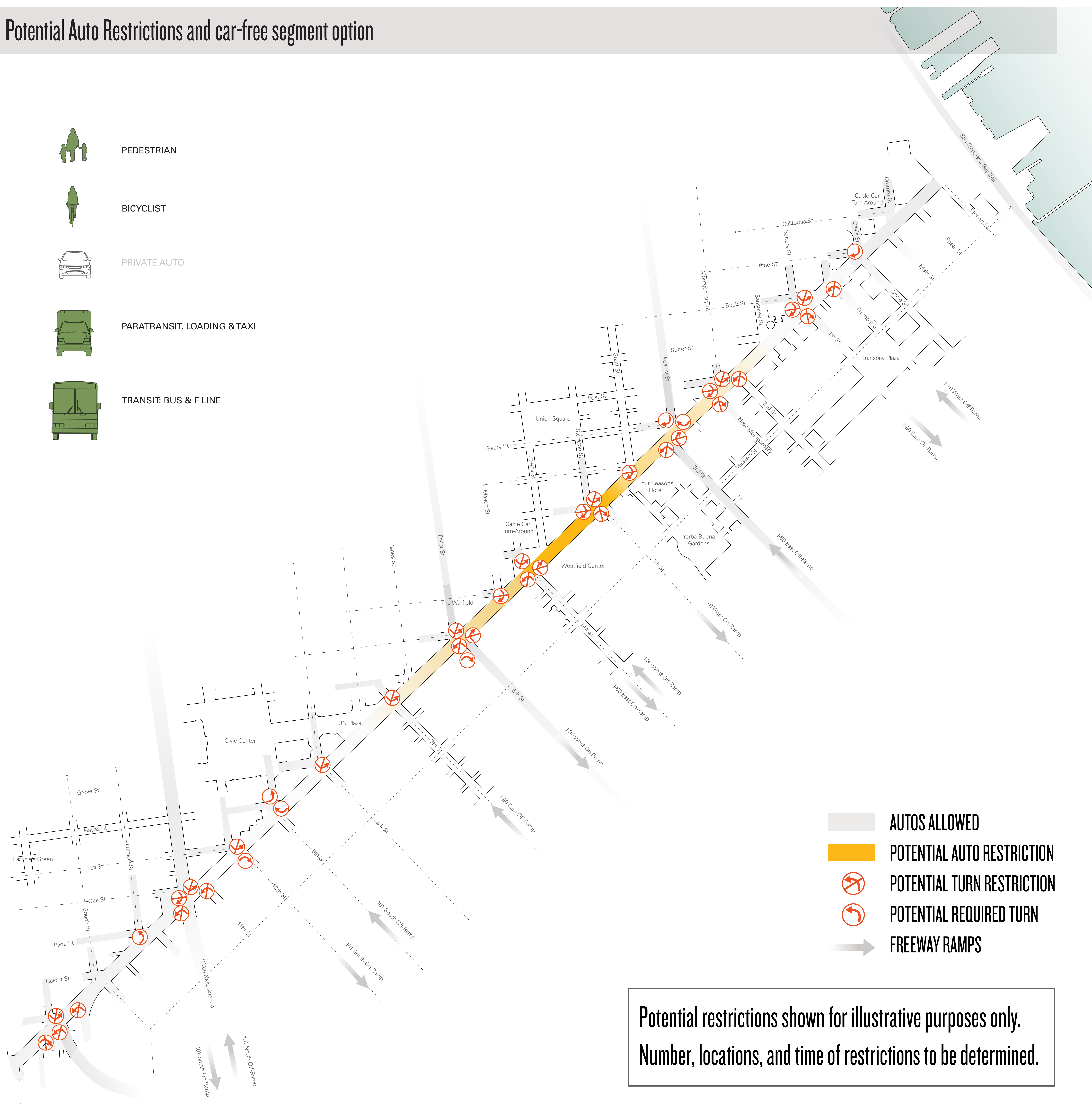
1. Introduces a car-free segment in area with the highest pedestrian, transit and cycling volumes.
